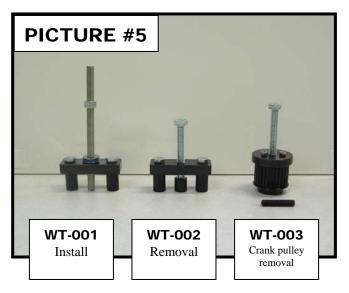
Note: Any tool that uses threaded rod or bolts; you should use lubricant on threads.
